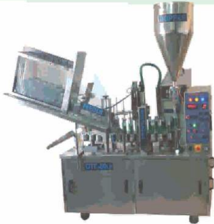
AUTOMATIC LINEAR LAMI TUBE FILLING MACHINE Output : 60 tubes per minute
